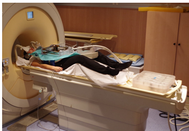
Fig. 5 The LPR V3 system installed on a volunteer in the MRI. The robot is on the subject's torso and the motor box is at the subject's feet on the MRI table
